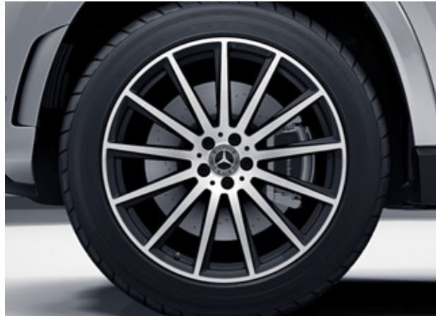
RPB 22" AMG alloy wheels (4) – multi-spoke design, painted black front: 285/45 tyres; rear: 325/40 tyres
