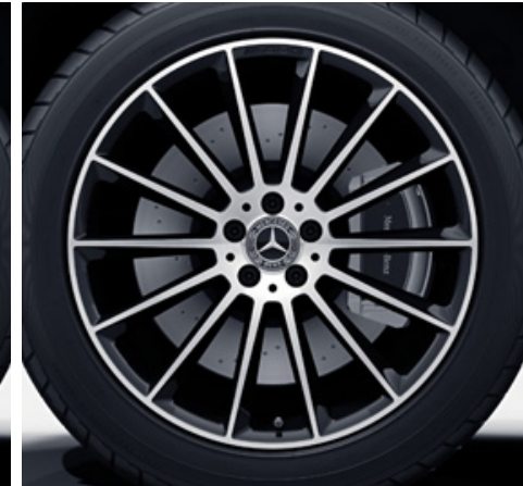
RWB 21" AMG alloy wheels (4) – multi-spoke light-alloy wheels painted in black with a high-sheen finish, front 275/45 tyres; rear: 315/40 tyres
