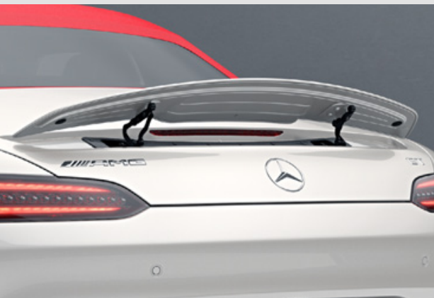
Rear aerofoil – electrically extending
