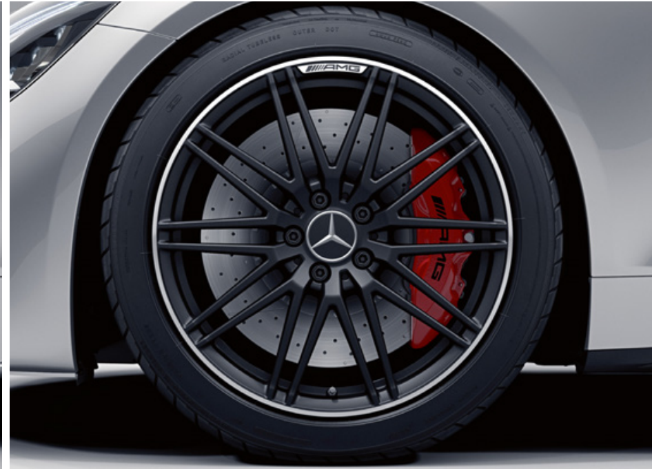
RXR 19"/20" AMG forged alloy wheels (4) – 10-twin-spoke design, painted matt black front 265/35 R 19 tyres; rear 295/30 R 20 tyres
