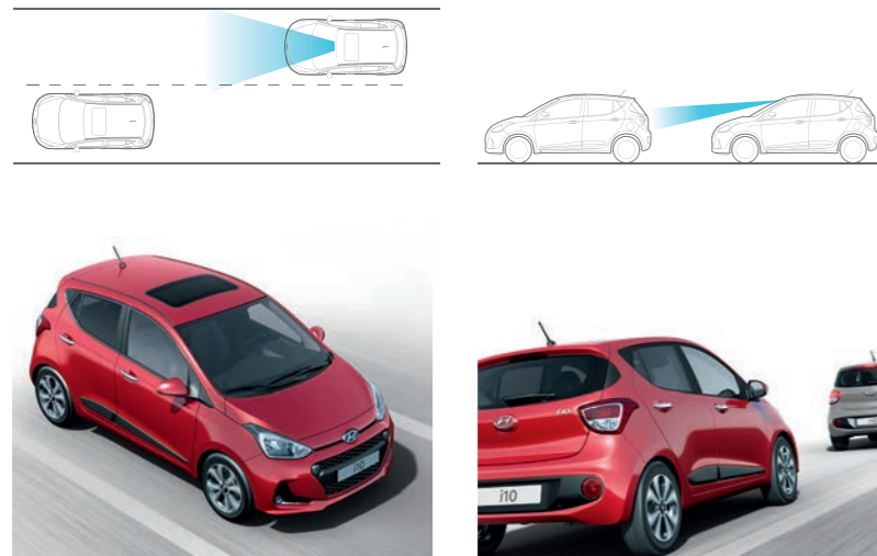
Lane Departure Warning (LDW) System: Warns you audibly and visibly of unintended departure from the traffic lane, when detected by the multi-function camera*.
