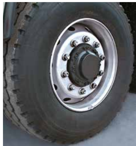
Front axle with hydrostatic wheel hub motors
