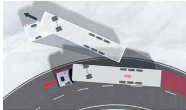
ESP compensatory braking when vehicle is oversteered
