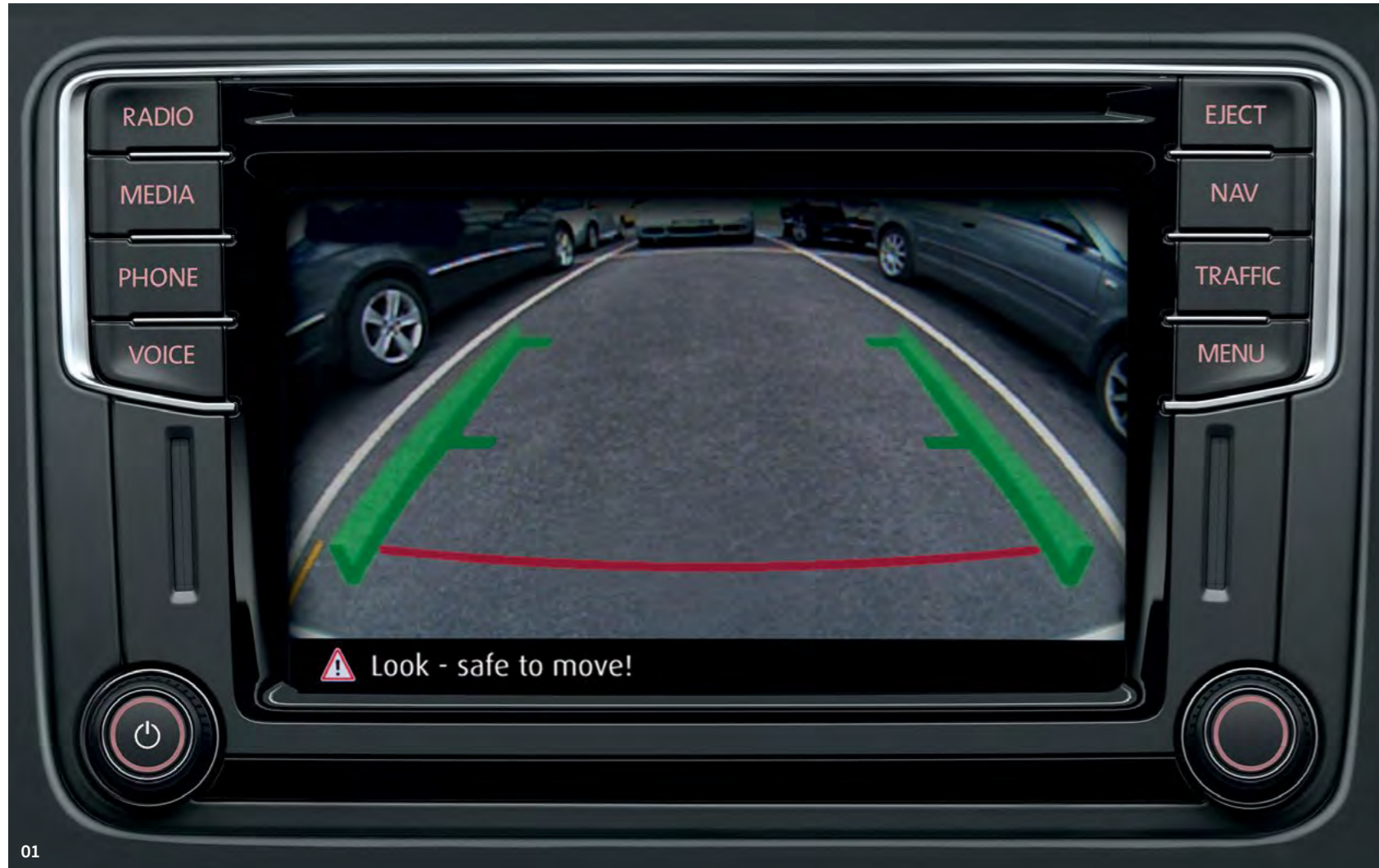
01 The rear-view camera helps you to reverse park, giving you a clear view to the rear of your vehicle via the vehicle's infotainment system display. Thanks to the high resolution detail, even small obstacles such as kerbs can be clearly recognised and avoided. Optional on SE Nav models.
