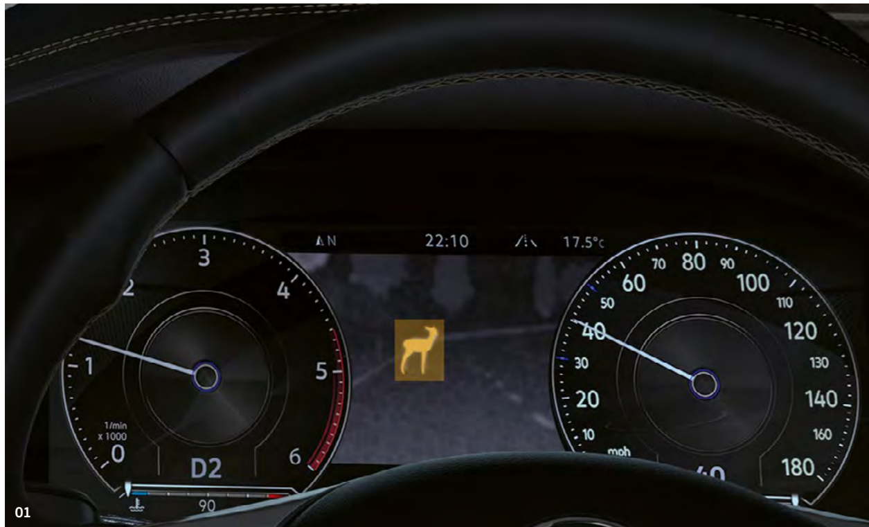
01 The innovative Night vision system 1 uses infrared beams to scan an area up to 130 metres ahead, detecting thermal radiation and projecting an image onto your Digital Cockpit or optional Head-up Display. If the situation is critical, the system will warn you and precondition the brake assistance systems, helping to keep you safe when driving at night. This is especially effective if your visibility is impaired by fog or rain, enabling you to see a person or animal ahead. Optional on all models.
